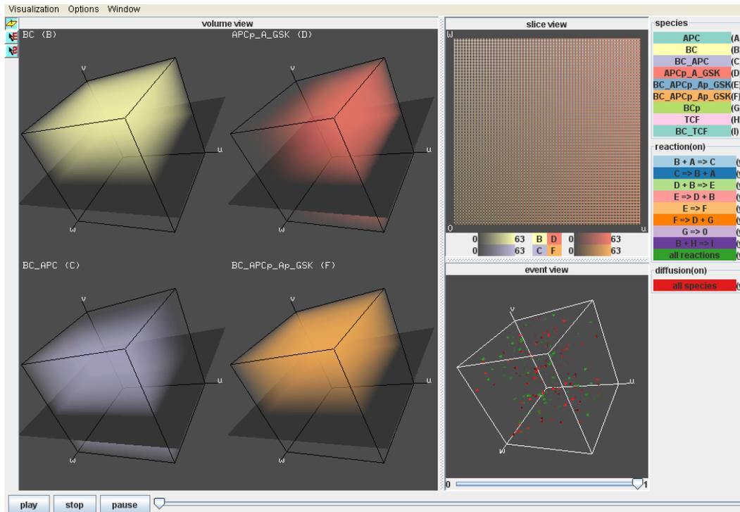
**Figure 5. The multiple view framework VioNeS, visualizing data at a single time point. In the state view (left), multiple univariate volumes are shown, each for a different state variable. The event view (bottom right) includes a sequence of previously occurred events in a univariate context, only separating diffusions and reactions. Their age is encoded by transparency. Additionally, a 2D slice view is included at the top right.**
