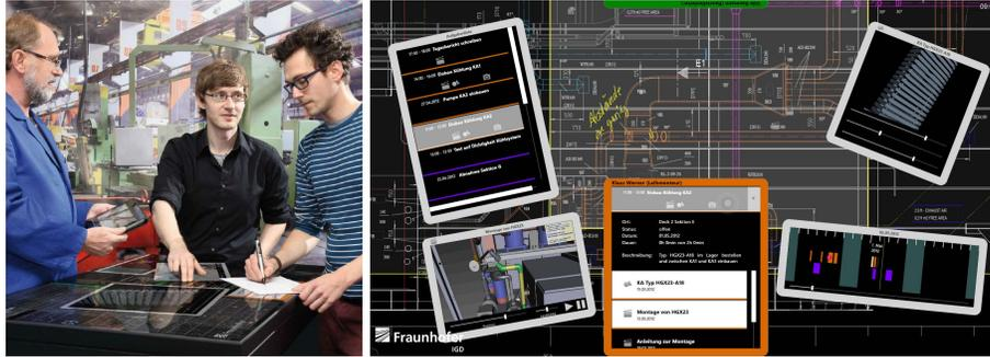
**Fig. 2.** An assembly team working collaboratively with Plant@Hand on a multi-touch table (left). Spatial and temporal contextualization of work orders in Plant@Hand (right). An underlying CAD drawing is used to provide context to the individual views, which are positioned at the place they refer to, e.g., a particular machine.
