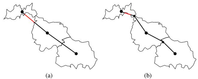
Fig. 5. Simple construction of geometrical path (a) without and (b) with border points. Red segments indicate violation of the inclusion requirement.
