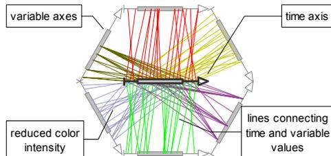
**Figure 2** A TimeWheel. Six variable axes are arranged circularly around an exposed centered time axis.
