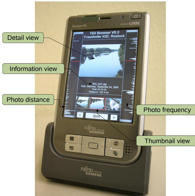
**Figure 2.** TiDi Browser on mobile device – The user interface of TiDi Browser comprises detail view, information view, and thumbnail view. Two time lines visualize photo distance and photo frequency, respectively. Both time lines serve as UI components to navigate in time.
