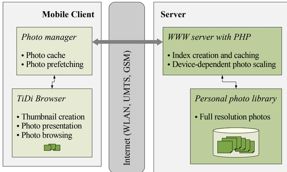
**Figure 3.** TiDi Browser client-server-architecture – On the client, TiDi Browser requests photos from a component called photo manger. The photo manager is responsible for the communication between the mobile device and the server. A WWW server with PHP provides access to the personal photo library located on the server.
